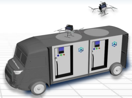
Mobile liquid hydrogen station
